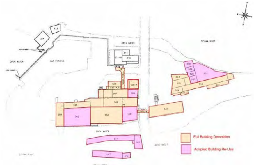
Figure 2: Buildings to be retained in Ottawa highlighted in pink.
